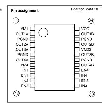
Since loads such as motors and coils are inductive, overshoots may occur on the powersupply voltage pin. Therefore, we recommend the connection of a roughly 10- $\!\mu F$  capacitor between the VM pin and GND.
